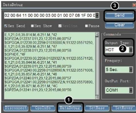
Fig 6-9 Setup of navigation output interface
