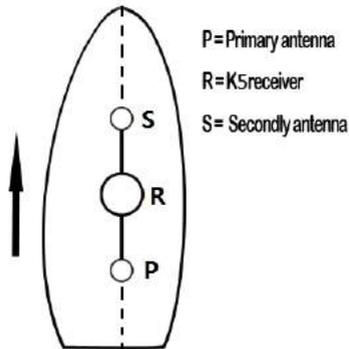
Fig4-7 Setup of dual-frequency antenna instruction
