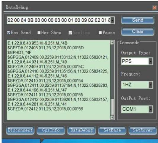
Fig 6-10 Setup of 1PPS output interface
