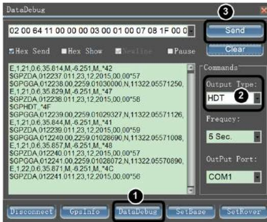
Fig 8-7 Setup of navigation output interface
