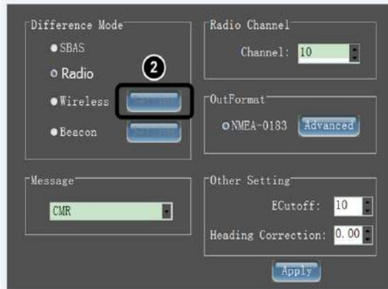
Fig 6-7 Wireless mode setup interface
