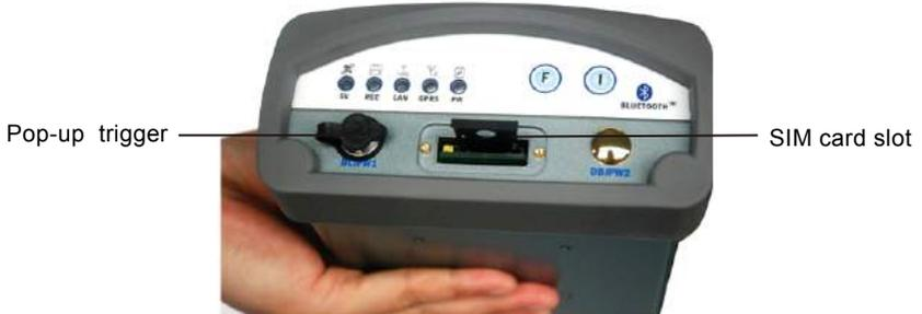
Fig 5-4 SIM card slot
