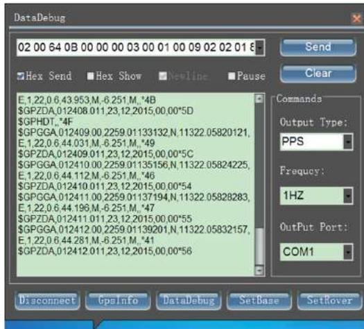
Fig 8-8 Setup of 1PPS output interface
