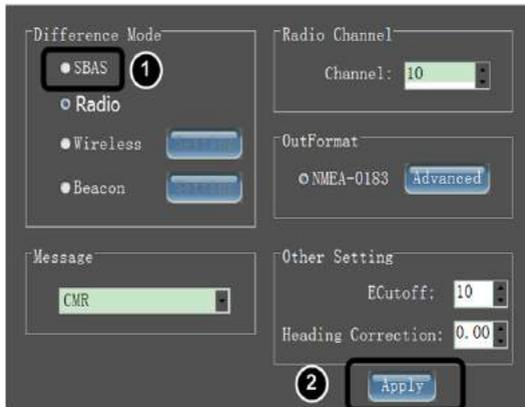
Fig 6-6 SBAS setup interface
