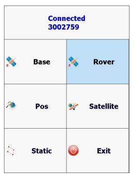
4. Go to Rover, set VRS parameters, then send V30 position to network.
