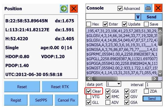
Tips: Once Hi-GNSS connected to V30, command has been send, NMEA output would be changed. In order to get clean NMEA message, first select Clear, click send; then select the options needed in DegiTerra, also click send. Next step, you can directly shut down Hi-GNSS, start your DigiTerra.
