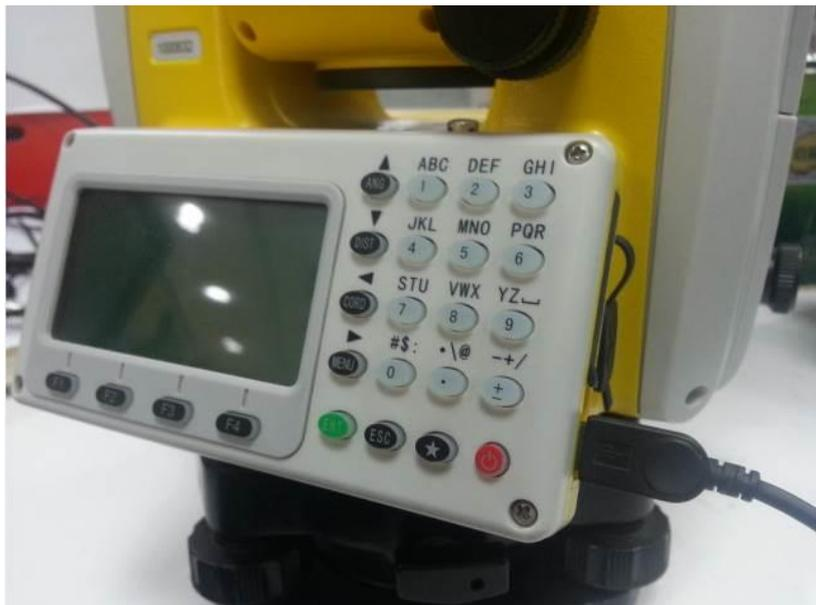
(2) Power on the TS (you will see the following interface)->Then turn to your PC there will display mobile disk inserted->open the mobile disk and copy data. Such as TEXT, MEA. Stored in the PROJECT folder.
